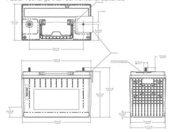
Length w/Rib: 12.9" Width: 6.77" Height w/Terminal: 9.25" 76lbs Weight: Terminal Type: Threaded Stud (Brass Pad) \*4 Years Free Replacement Warranty: From Factory Defect (car, light truck and SUV) \*3 Years Free Replacement from Factor Defect (Marine and Recreational vehicles).
